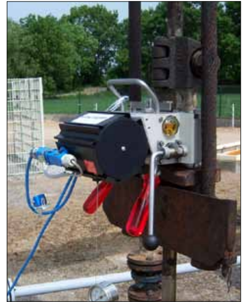
Installation of the Dynamometer DYC
