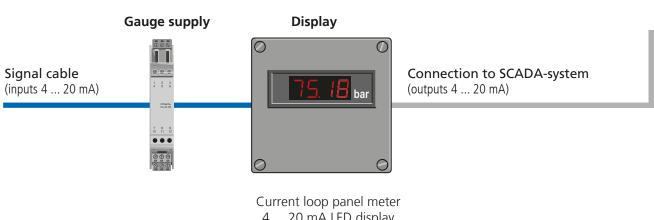
Current loop panel meter 4 ... 20 mA LED display without power supply intrinsically safe EEx ia/ib IIC T6 (T5)
