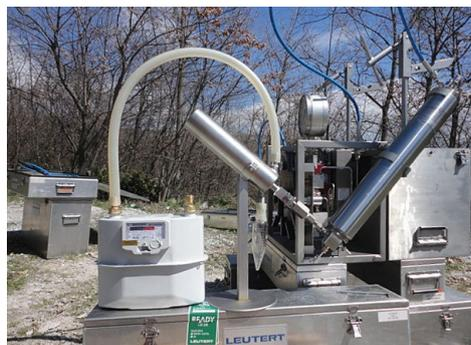
*GOR in black-oil from samples taken via Leutert Bottomhole Sampler in combination with the BSW&G flasher*
